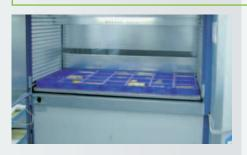
The extractor device delivering the requested tray to the access opening or back to a free storage location within the device at fast speeds. At the push of a button or scan of a barcode.
