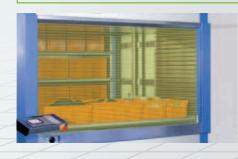
Side walls of the access opening are equipped with L-profiles. These enable the positioning of multiple trays in the access opening (Double access handling) as well as individually adjusted working positions for each individual operator depending on their physical height.
