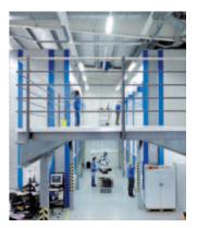
Vertical Lift Modules can go through several floors with up to 6 access openings placed on the front or rear side of the unit. A mezzanine floor can be installed to enable operation on several levels at the same time (with loading at one level or side and retrieval at the other).
