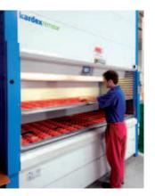
Thanks to the 'Double access handling' option it is possible to use two work levels in the access opening. A tray is transported into the first work level in the access opening and the shutter door closed. While articles are stored or removed, the next tray is being retrieved and kept in a waiting position behind the access opening.
