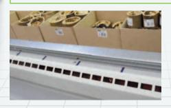
To improve operators' productivity, throughput and accuracy levels Kardex Remstar offers several integrated pick-to-light technologies to match most organisations' needs and applications. Shuttle XP's can be equipped with position indicators, light pointers and confirmation bars in the access opening.
