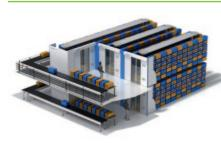
For more comprehensive systems, multilevel stations can meet the requirements of a great variety of different material flow strategies. Multilevel stations – two or three Horizontals stacked one above the other - allow for picking and putting on different floor levels. Each level operates independently; with seperate access and picking stations located at each floor level and on each platform. For uninterrupted material flow between the different levels, conveyors can be used to transport items.
