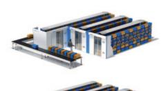
Triple stations or quadruple stations are recommended for applications with a wide range of items that require frequent access - the layout is usually L-shaped.
